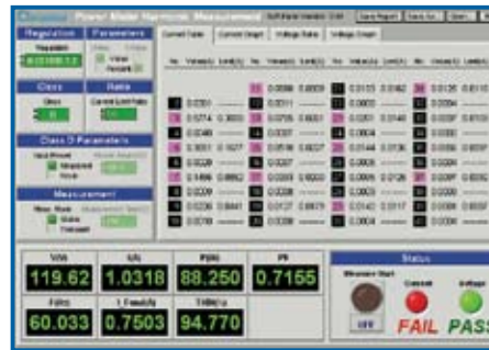
IEC 61000-3-2 Current Harmonic Test
